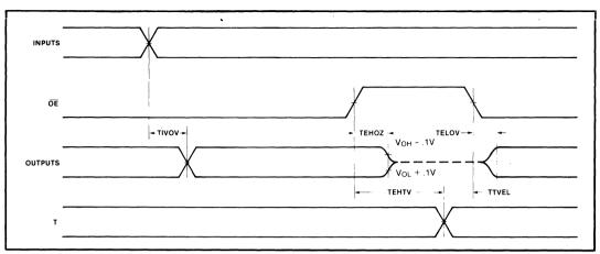
NOTE: 1. All timing measurements are made at 1.5V unless otherwise noted.
